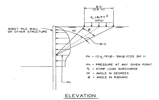
LATERAL PRESSURE DUE TO STRIP LOAD
