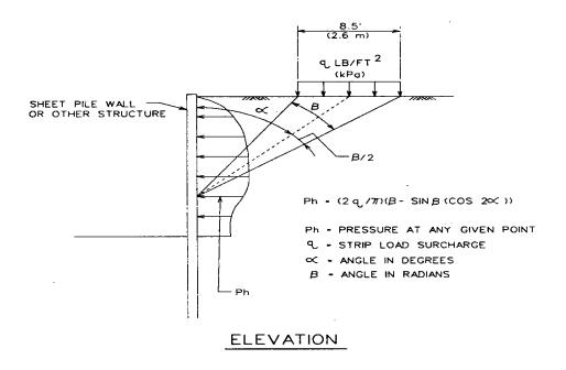
LATERAL PRESSURE DUE TO STRIP LOAD
