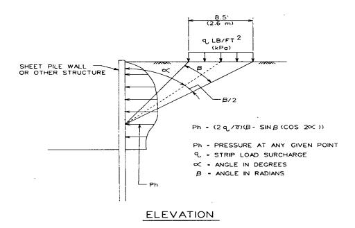
LATERAL PRESSURE DUE TO STRIP LOAD
